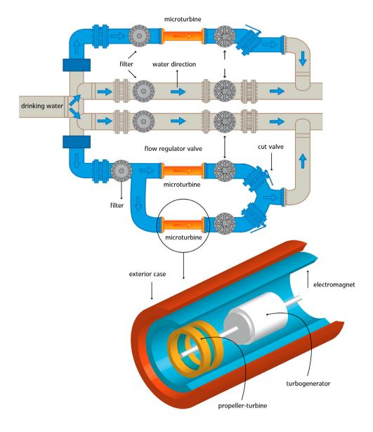
This project consists of harnessing existing flows and over-pressures detected on the network through installing micro-turbines for power generation. With this project Canal Gestión will have, from 2016, 1 extra GWh of renewable energy, without altering the quality of the water supplied in any way.
