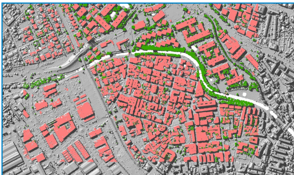
Figure e. Observation and detailed modelling techniques, based upon the use of hyperspectral sensors and laser
